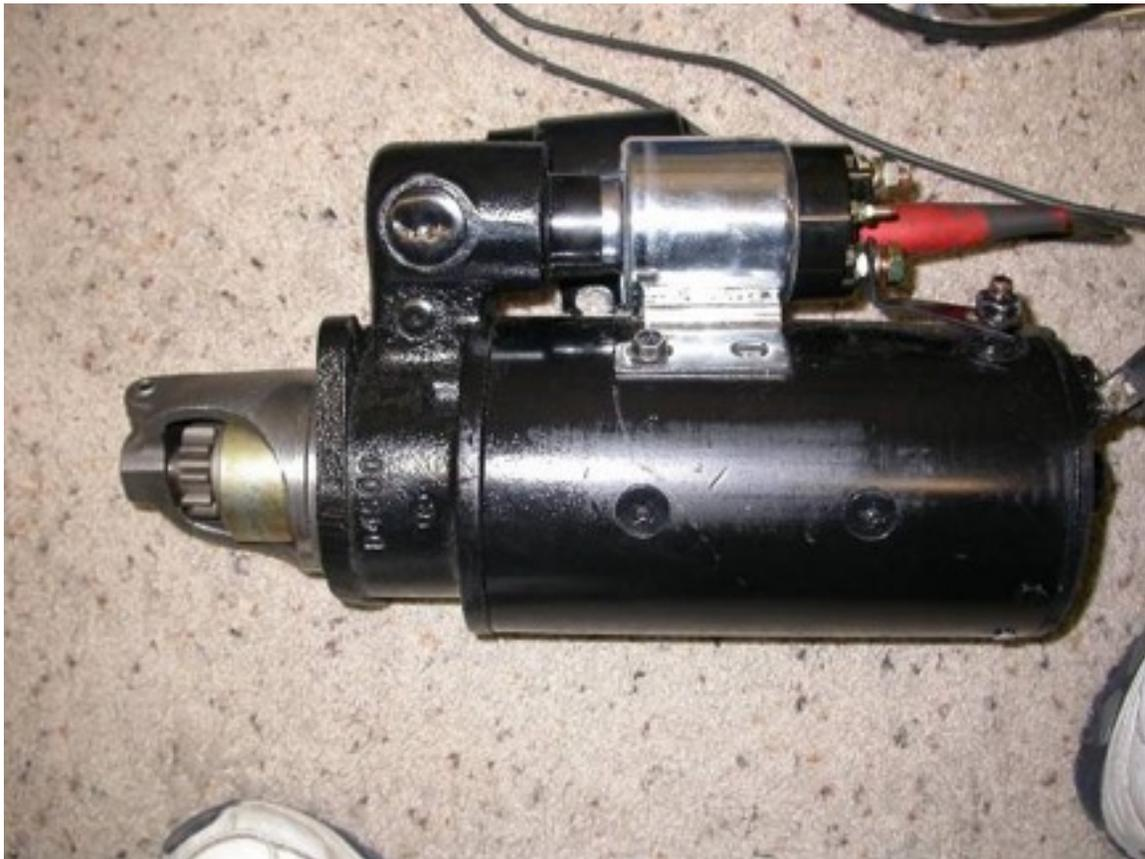
2. Install just the 2 solenoid mounting screws closest to the lever housing, and leave them about 1 to 2 turns loose.
